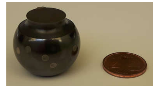
Curved sample with measuring spots beside a 2-cent-coin for a size comparison
